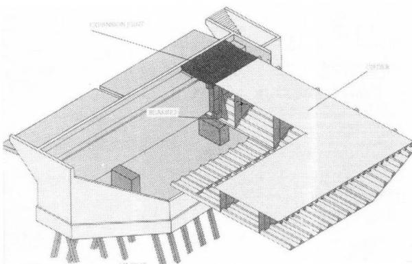
Fig. 4.4 Farø Bridges. Abutments
