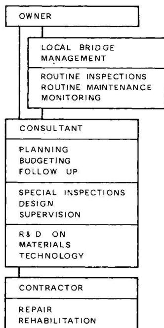
Fig. 7.1 Diagram of typical maintenance organization
