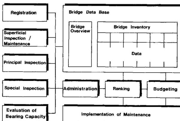
Fig. 8.1 Diagram Bridge Management System
