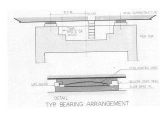
Fig. 4.4 Farø Bridges. Abutments
