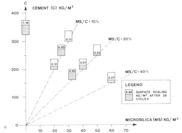
Fig. 5.2 Freeze-thaw tests. Concrete with different amounts of microsilica and no air entrainment
