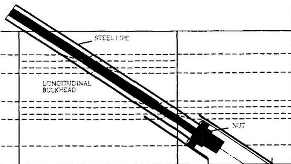
Fig. 4.2 Farø Bridges. Stay Anchorage in Girder
