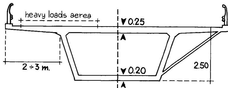
DOUBLE BOX GIRDER - Steel/concrete or P.R.C. with anti roll over
