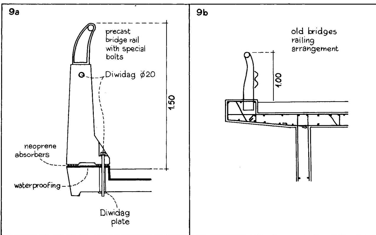
impact strength of these devices is a mixed function of beam and bracket, based on a dywidag Ø 20 horizontal bar and attachments, of a strength varying according to the reinforcing present in the structure, at the foot of the wall, which has a New Jersey profile. An additional steel handrail or the wall itself extended to a height of 1.70 m from the road surface comprises the upper part of the structure. In cases of collision, maintenance is immediate, as the element can be replaced in minutes.
