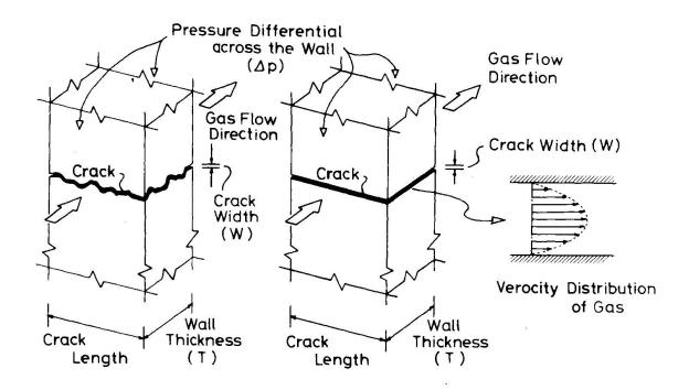
Fig.4 Idealization of crack and gas flow
