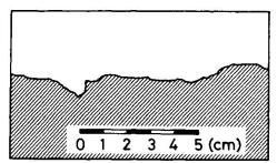
Fig.6 The crack surface of the concrete A
