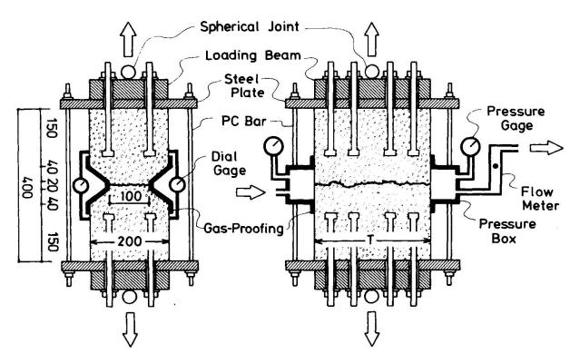
Fig.3 Specimen and testing set up
