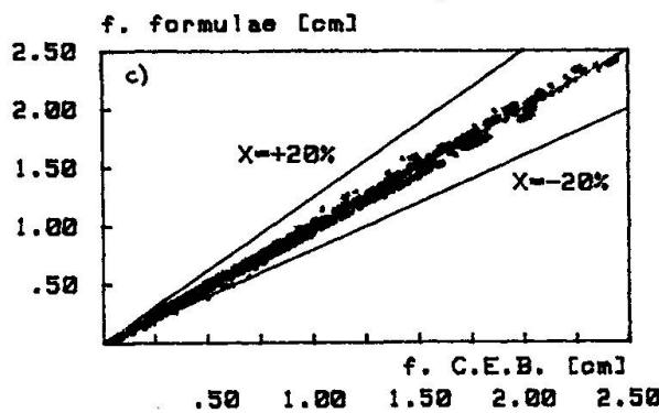
Fig. 4 Comparison of computed short and long-term deformations using simplified formulae and CEB method. a) hinged-hinged beams. b) fixed-hinged beams. c) fixed-fixed beams.
