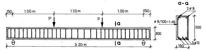
Fig. 1. The test beams
