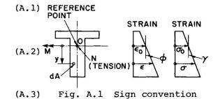
where A, B and I are the area, its first and its second moment about an axis through 0;  $\sigma$  is the stress at 0 and  $\gamma$  is the slope of the stress diagram. Equations A.3 can be used to determine the stress resultants N and M for a specified stress distribution. When N and M are given, the strain at 0 and the curvature may be determined by:
