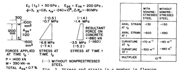
Fig. 3 Stress and strain in a member in flexure
