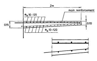
Fig. 2 Reinforcement of the balcony slab
