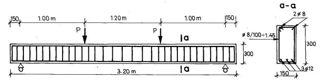
Fig. 1. The test beams
