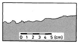
Fig.8 The crack surface of the concrete C
