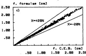
Fig.4 Comparison of computed short and long-term deformations using simplified formulae and CEB method. a) hinged-hinged beams. b) fixed-hinged beams. c) fixed-fixed beams.
