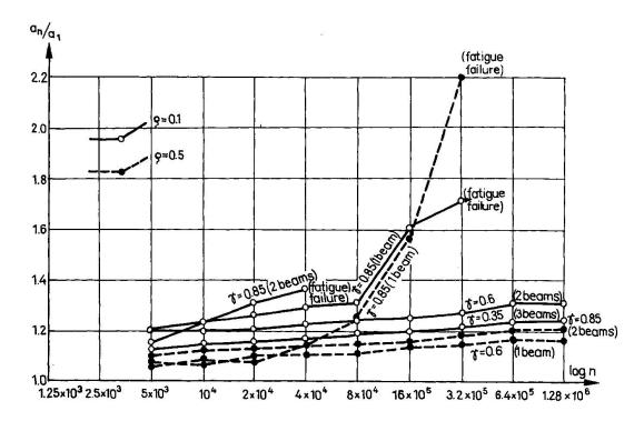
Fig. 2. The ratios of the deflections measured after n cycle (a<sub>n</sub>) to the deflections measured after the first load cycle (a<sub>1</sub>)
