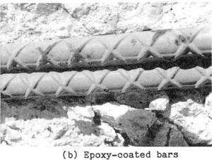
Fig. 6 Visual appearance of bar and concrete surfaces after test
