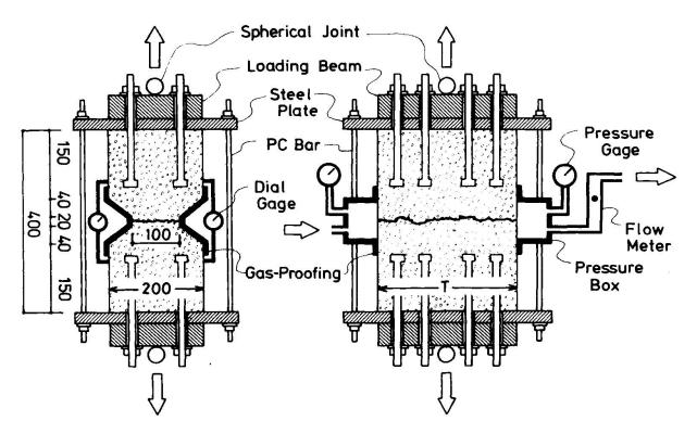
Fig.3 Specimen and testing set up
