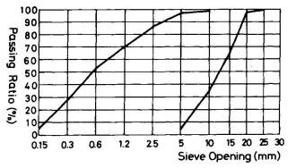
Fig.1 Sieve analysis curve of the concrete A
