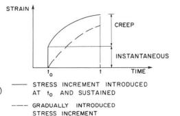
Fig. 4 Time variation of strain due to a stress increment
