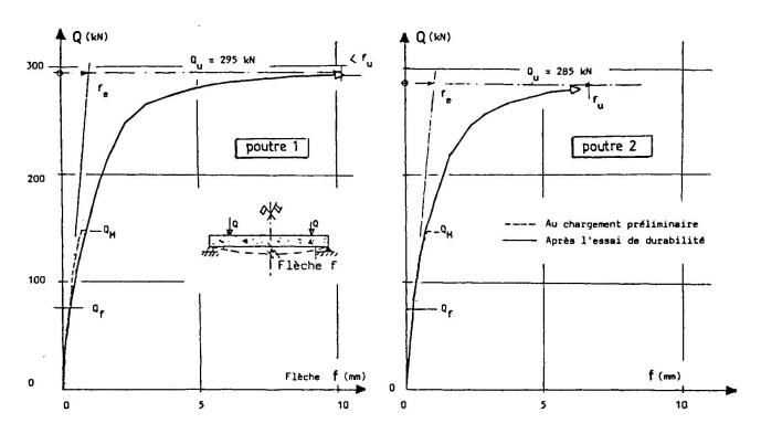
Fig. 4 Diagrammes "flèche f-charge Q"
