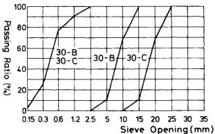
Fig.2 Sieve analysis curve of the concrete B and the concrete C
