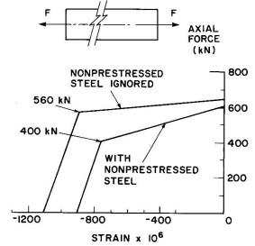
Fig. 2 Strain due to axial force applied at time t in the tie of Fig. 1
