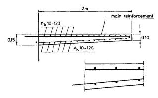
Fig. 2 Reinforcement of the balcony slab
