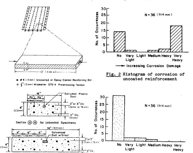
Fig. 1 Durability specimen details
