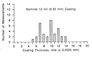
Fig. 7 Variation in coating thickness 36 mm bars
