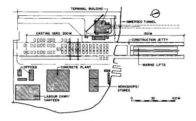
Fig. 3 Lay-out of work site
