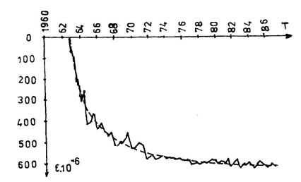
By the correlation function for Q = 615 was ascertained, that A = 22,25 and B =-679. The standard deviation s = 26,95; the theoretical deformation after 20 years Y<sub>20</sub>= -604.10 and after 100 years Y<sub>100</sub>= -646.10 .Very similar result we received also using the function Y = A.VT + B.T.
