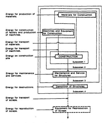
Fig. 2 Flow chart of energy consumption, in construction
