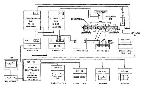
Fig.5 Diagram of the Online-Hybrid System
