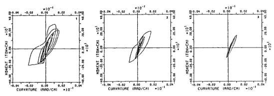
Fig.7 Experimental Moment-Curvature Relation of the Specimen in Every 10 Seconds of Earthquake Response
