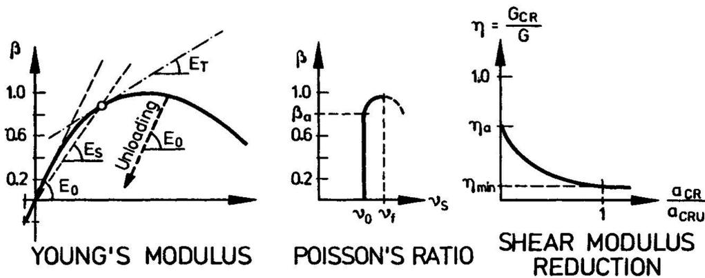
Figure 1: Modified triaxial constitutive assumptions for concrete resulting from [6]
