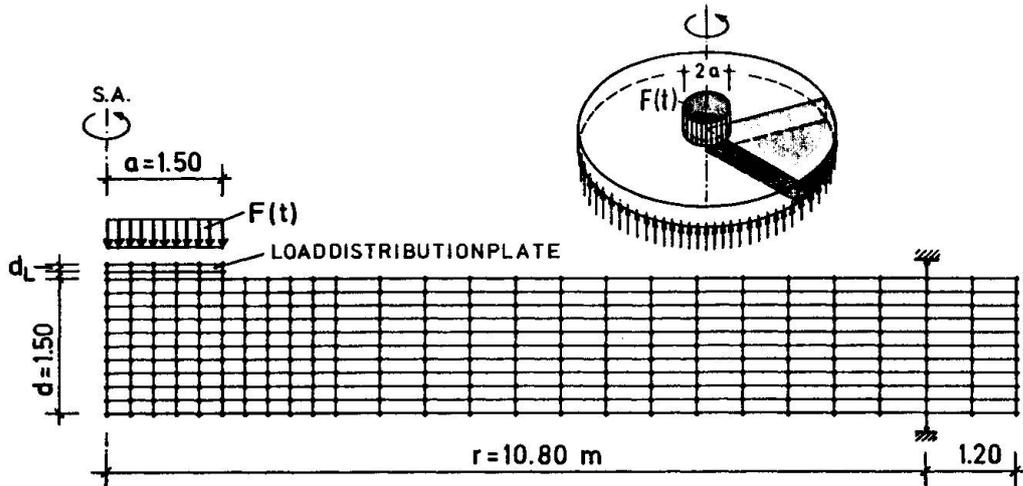
Figure 3: Discretisation of the axisymmetric slab
