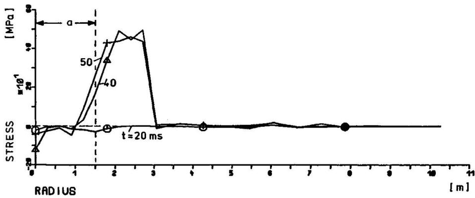
Figure 9: Stresses in stirrups with 'rigid' load introduction
