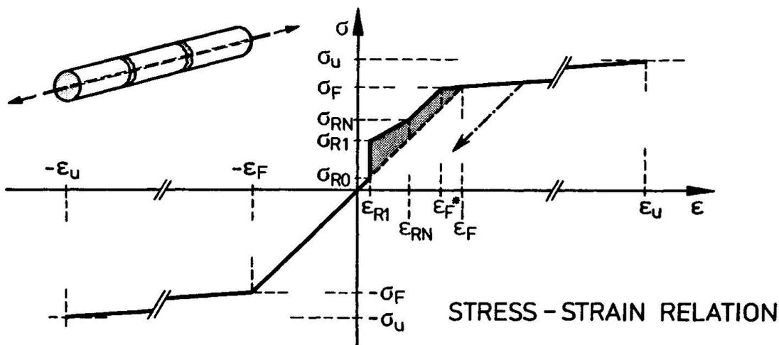
Figure 2: Constitutive assumptions for reinforcement including 'tension-stiffening'
