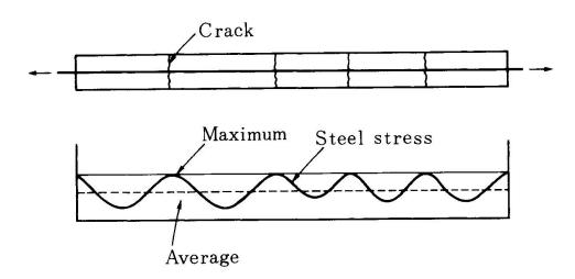
Fig.19 Stress distribution of reinfrocement in cracked concrete
