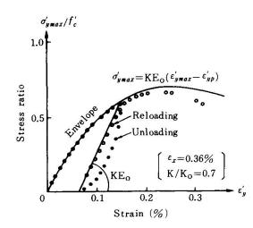
Fig.13 Modified Maekawa model versus experimental result [23]
