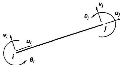
Fig.4 Degrees of freedom of a beam element
