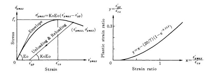
Fig.8 Maekawa model for compression [10] Fig.9 Plastic strain in terms of a function of the maximum compressive strain [10]
