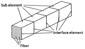
Fig.3 Division of a beam element
