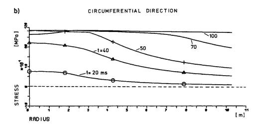
Figure 8: Stesses in bending reinforcement a) radial direction, b) circumferential direction
