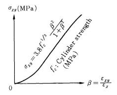
Fig.15 Shear transfer mechanism
