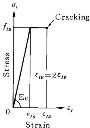
**Fig.3** Stress strain relation of concrete for tension
