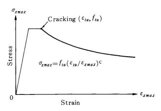
Fig.3 Stress strain relation of concrete for tension
