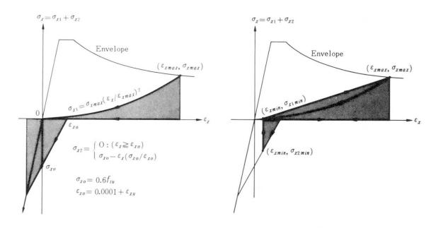
Fig.6 Tension stiffening model for unloading [22]
