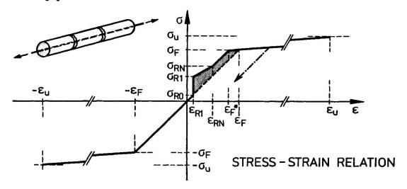
Figure 2: Constitutive assumptions for reinforcement including 'tension-stiffening'
