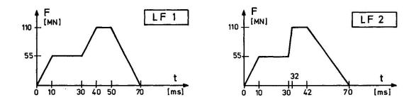
Figure 4: Applied load-time functions
