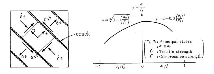
Fig.1 The coordinates for cracked concrete
