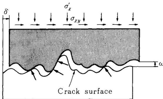
Fig.15 Shear transfer mechanism
