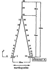
Fig.15 An RC tower model
