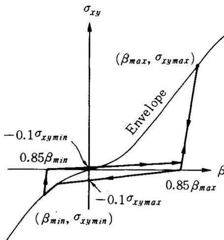
**Fig.17** Shear transfer model for unloading and reloading
