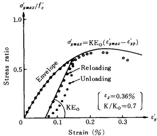
Fig.13 Modified Maekawa model versus experimental result [23]
