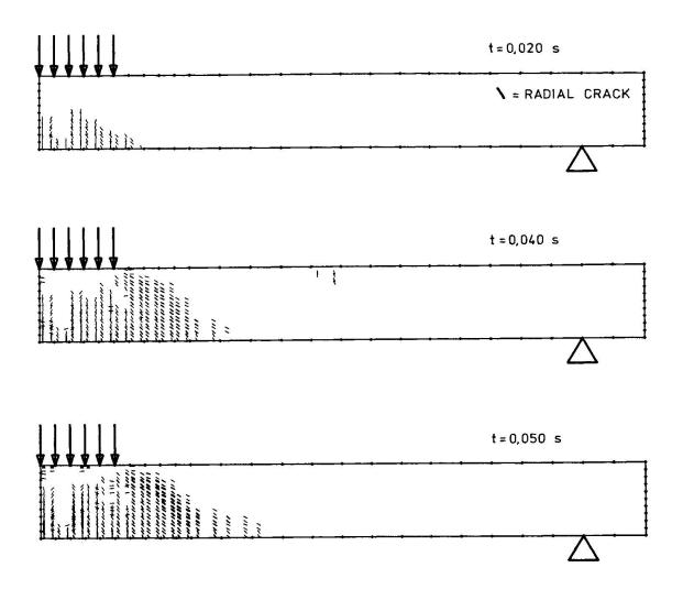
Figure 6: Developement of radial cracks of the 1,50 m thick slab
