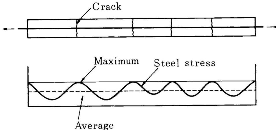
Fig.19 Stress distribution of reinforcement in cracked concrete
