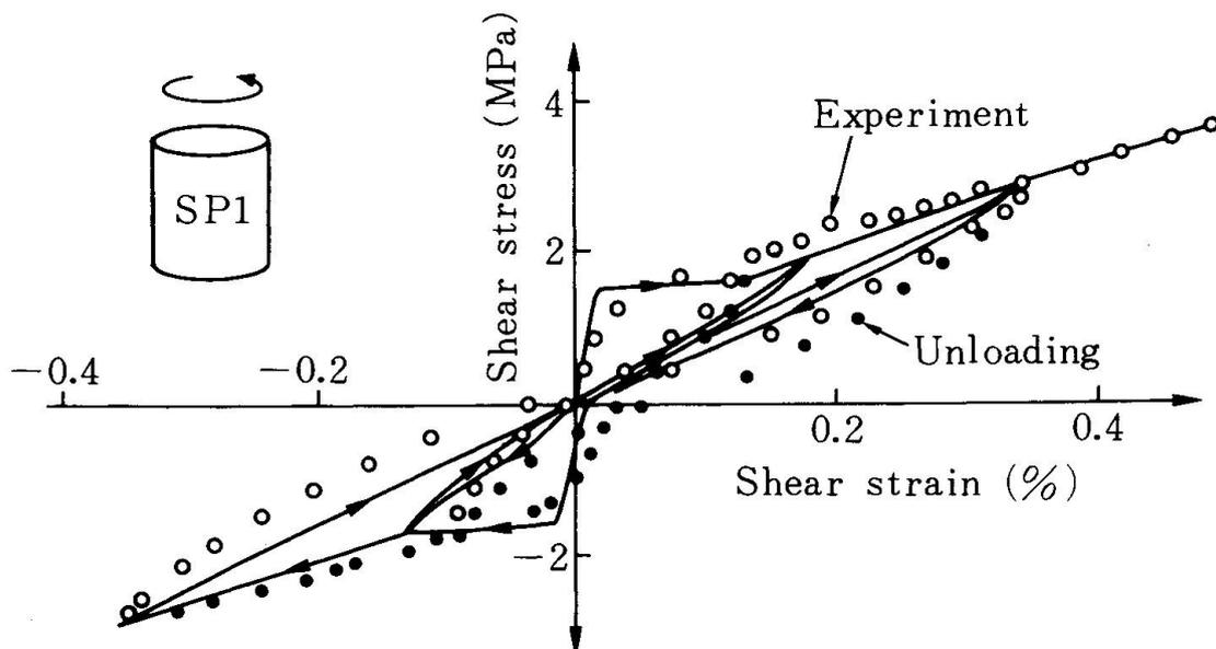
Fig.24 Comparison of the calculations with the experimental results by Yoshikawa et al. for reversed cyclic loading
