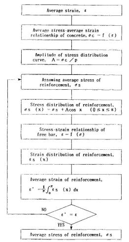
Fig. 7 Calculate procedure to obtain average stress-strain relationship of steel bar in post yield range
