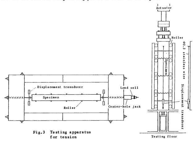
Fig. 4 Testing apparatus for reversed loading
