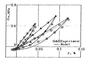
Fig.10 Relationship between ocb and average strain
