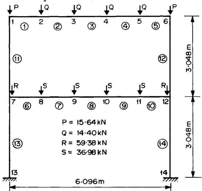
The El Centro 1940 S00E ground motion, multiplied by a factor  $\lambda$ , was applied to the two-storey frame. The factor  $\lambda$  can be compared to the load factor for static loading conditions.
