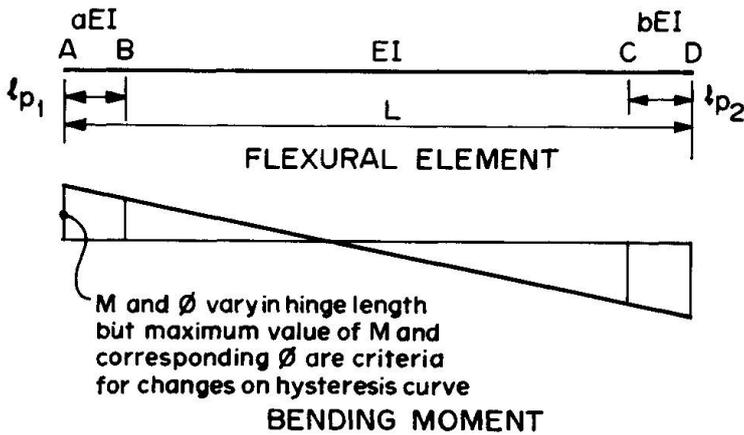
Fig. 1. Plastic-softening hinges at end of flexural element.
