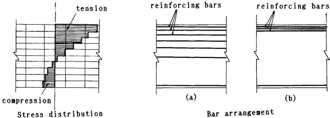
**Fig. 5** Reinforcing bar arrangement example according to plane stress analysis
