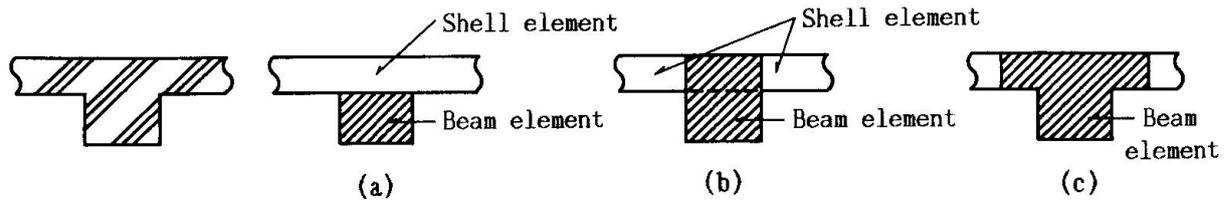
**Fig. 3** Modeling of beam and shell elements
