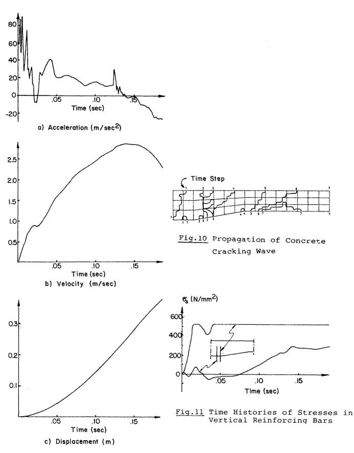
Fig.9 Time History Response of Tunnel Midspan Section
