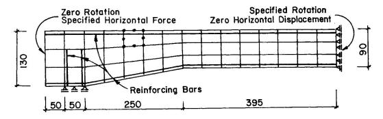
Fig. 4 Finite Element Model of Tunnel Roof
