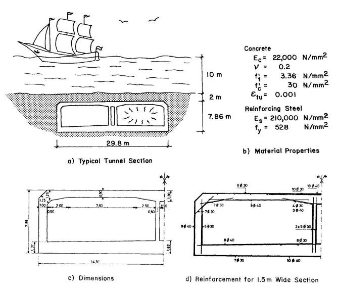
Fig.1 Typical Tunnel Section
