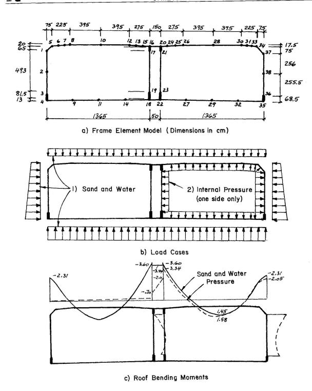
Fig. 3 Linear Elastic Static Analysis of Frame Element Model
