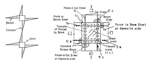
Fig. 1 Moment diagram of frame under seismic force
