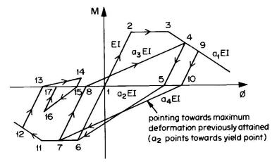
Fig. 2. Hysteresis model for plastic-softening hinges.
