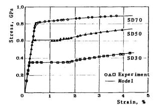
Fig.2 Stress-strain relationships of steel bars
