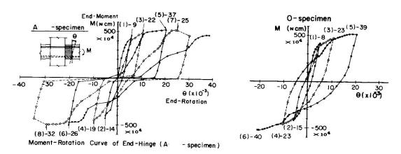
Fig. 8 Analytical moment-rotation curve of end hinge O-specimen
