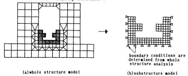
Fig. 1 An example of substructure model
