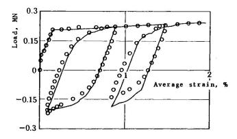
Fig.12 Comparison of analytical and experimental results of loadaverage strain relationship in post yield range
