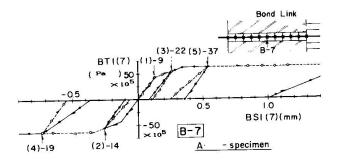
Fig. 10 Bond stress-slip histories in A-specimen
