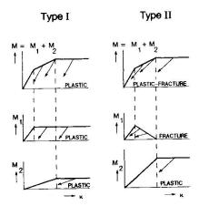
Fig. 2 Decomposition of constitutive model in two components. Left: two elasticplastic springs representing the plastic model. Right: one elastic-fracture spring representing the plastic-fracture model.
