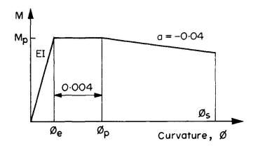
Fig. 5. Hinge properties for example frame.
