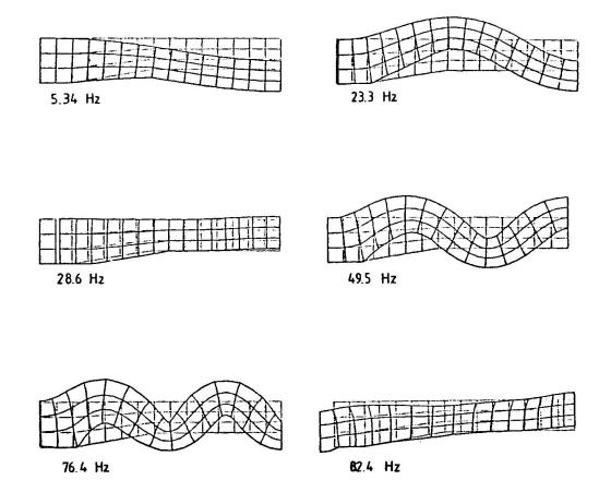
Fig.7 First Six Modes and Frequencies of Finite Element Model
