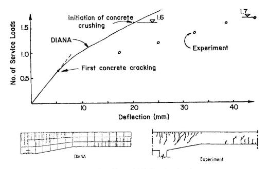
Cracking at 1.7 Service Loads
