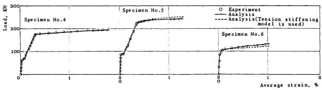
Fig. 8 Comparison of analytical and experimental results of load-average strain curve
