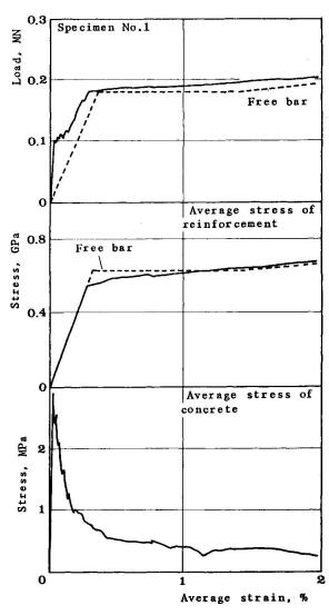
Fig.6 Load vs average strain and average stress-strain relationships of steel bar and concrete
