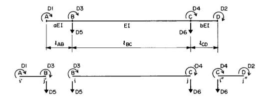
Fig. 3. Assembly of flexural element.
