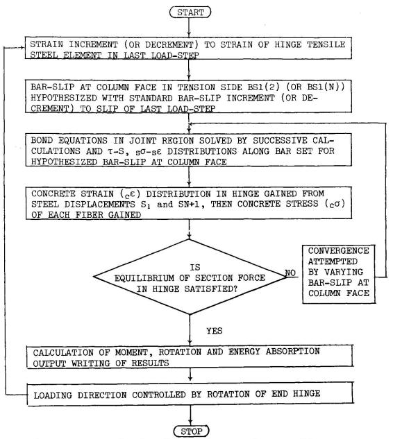
Fig. 5 Flow diagram for computer program
