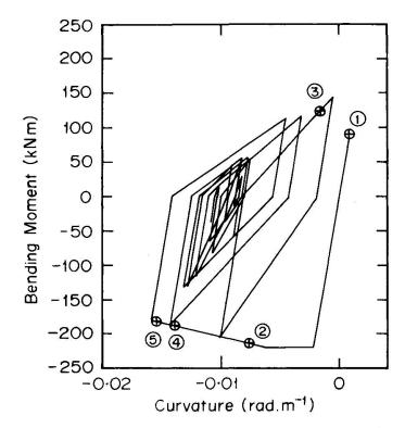
Fig. 7. Bending moment vs. curvature, member no. 10, node no. 12.
