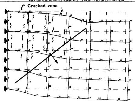
Figure 5 Example of plane stress finite element mesh and distortions for a/d ratio of 1.
