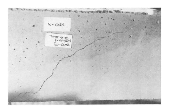
Figure 3 Photograph showing diagonal cracking for beam unreinforced for shear with a/d ratio greater than 2 just prior to ultimate shear collapse.
