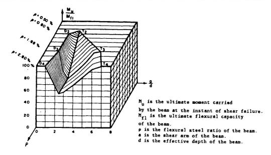
Figure 1 Kani's valley of diagonal failure for mild steel, 300mm deep, RC beams subjected to two-point loading.
