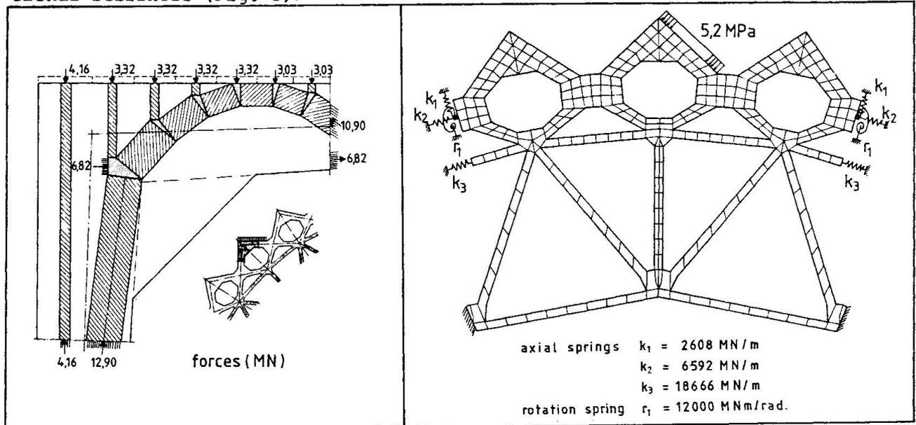
Fig. 7 Plastic lattice model part of triangular projection (load = 5.2 MPa;  $\gamma_m = 1.3$ )
