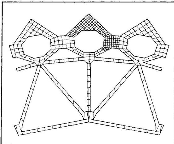
Fig. 10 Computer model for non-linear analysis
