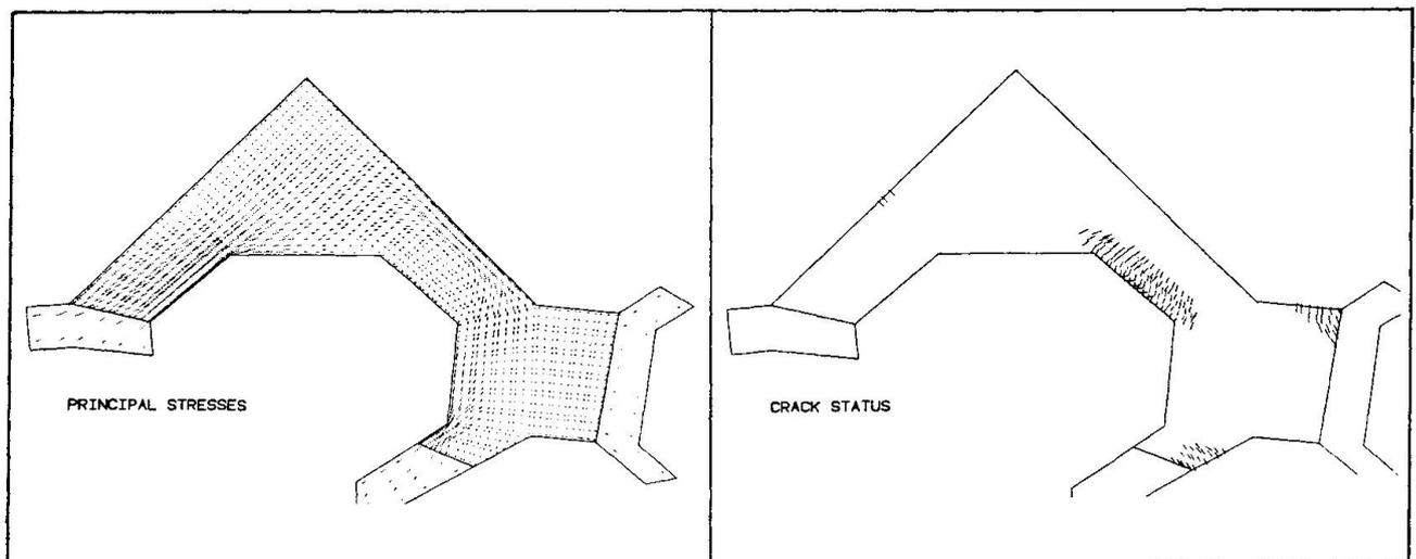
Fig. 12 Results after minimum design ice loading (5.2 MPa)
