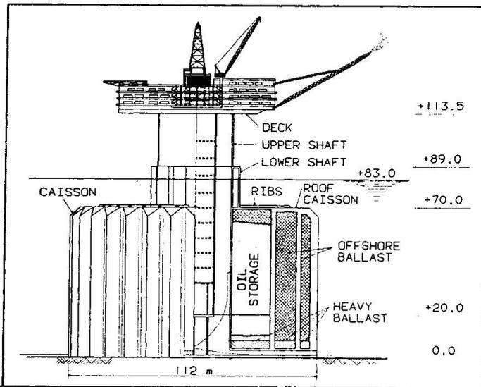
Fig. 1 Selected concept; view and vert. cross section
