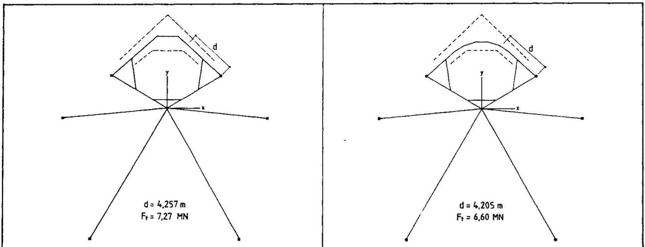
Fig. 15 Alternatives plane frame model of triangular projection
