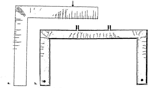
Fig. 10. a. Cracks at failure
