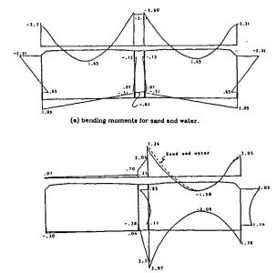
Fig. 22. Bending moments obtained with frame element model
