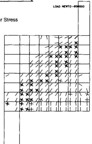
Fig. 11. Diagonal Strut Compression Failure
