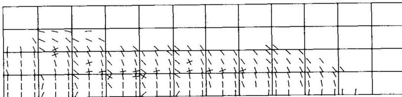
Fig. 10. Detection of Beam Shear Failure by Cracking
