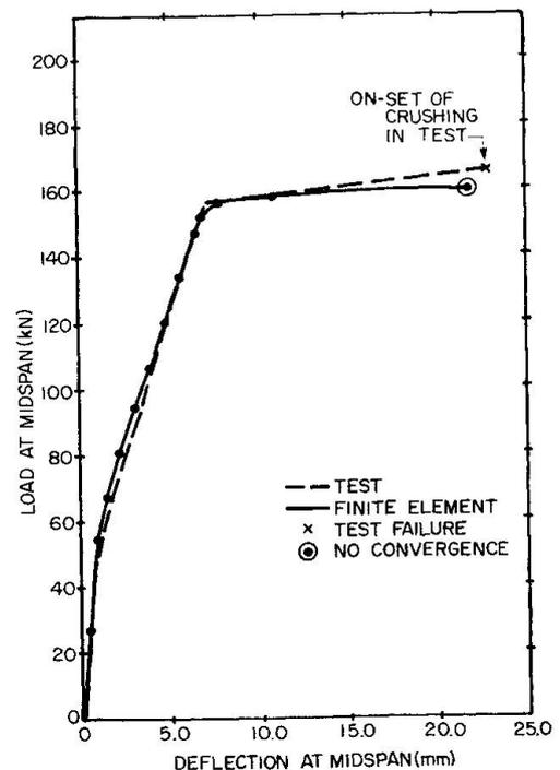
Fig. 5. Comparison with Tests for Beam Flexural Failure
