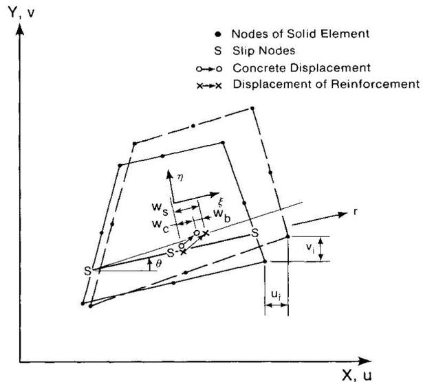
Fig. 1. Displacements for Embedded Bond Elements
