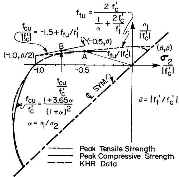
Fig. 3. Peak Strength Envelopes in Biaxial Stress Space
