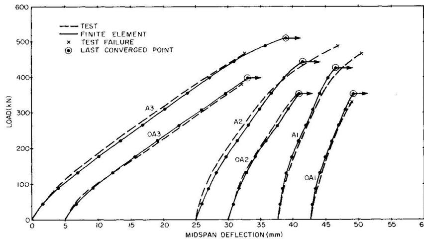
Fig. 6. Comparison with Tests for Beam Shear Failures
