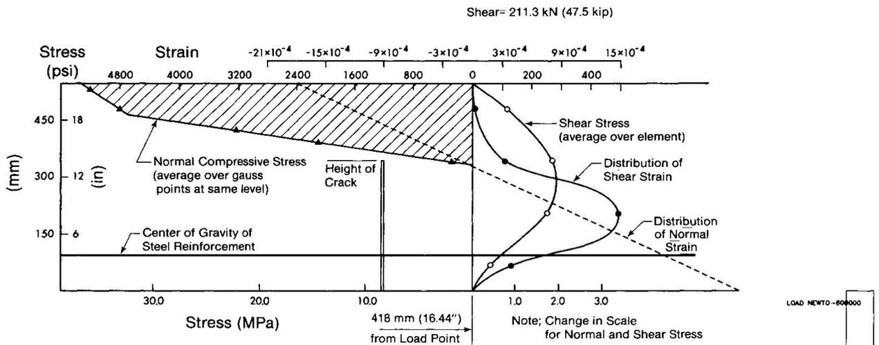
Fig. 9. Detection of Beam Shear Failure by Shear Strain
