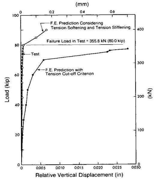
Fig. 8. Detection of Beam Shear Failure by Thickening
