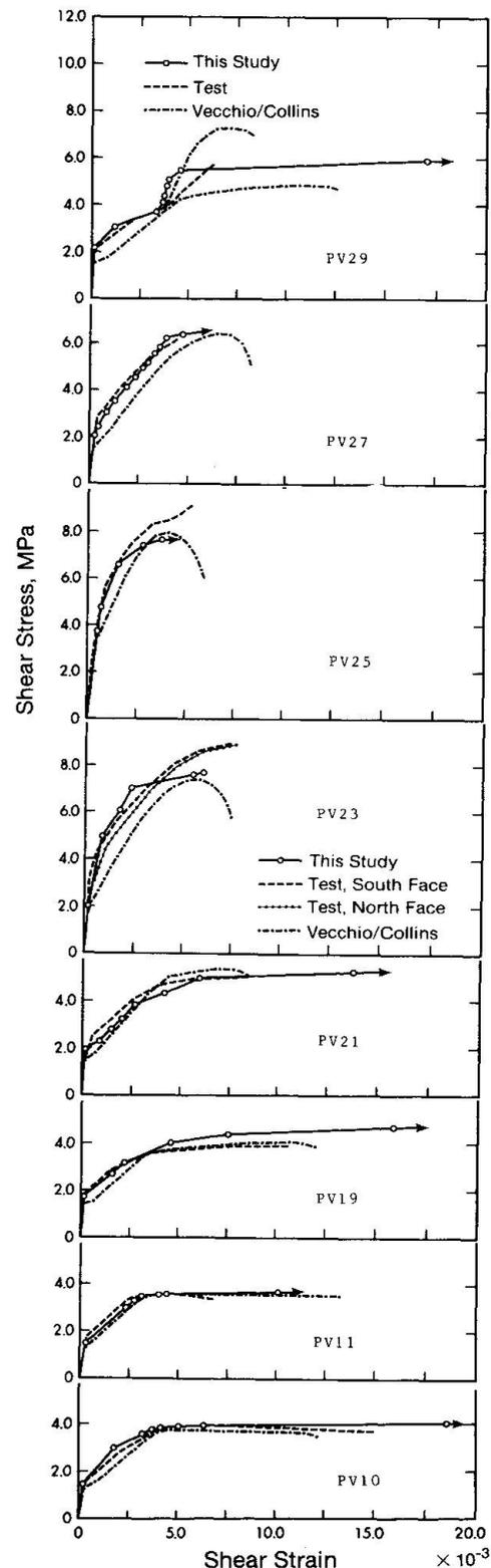
Fig. 4. Comparison with Tests for Vecchio/Collins Panels
