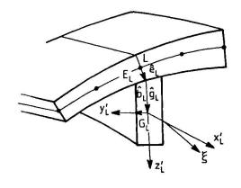
Fig.1 Geometry of the eccentric beam element
