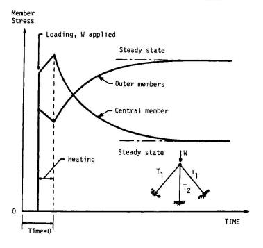
Fig. 6. Variation of member stresses with time in heated pin-jointed structure
