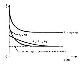
Fig. 2. Dependence of Energy Dissipation Rate on elastic and viscous parameters of Maxwell model. Note: for concrete,  $\eta = 1/\phi(T)$ .
