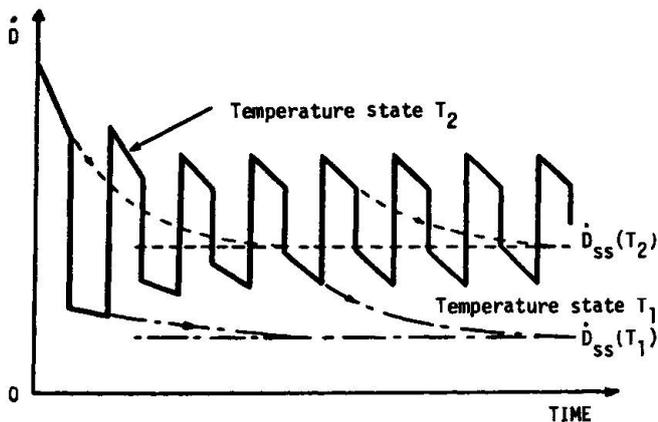
Fig. 4. Energy Dissipation Rate - Time behaviour under cyclically changing temperature states.
