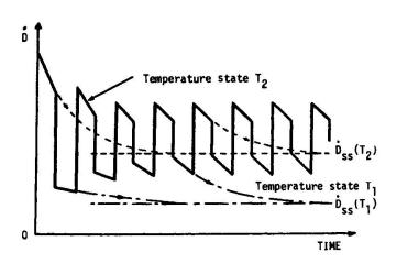
Fig. 4. Energy Dissipation Rate - Time behaviour under cyclically changing temperature states.
