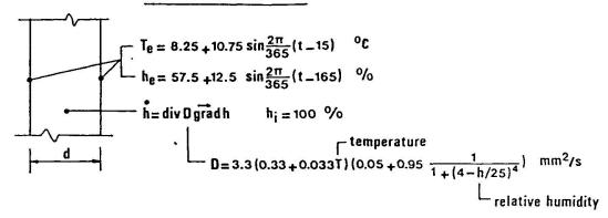
$\frac{\text{Fig. 12}}{\text{of element 5 of the cross section.}}$  Diffusion equation and boundary conditions used in the drying analysis
