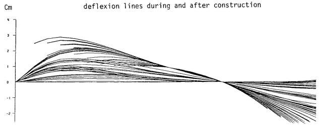
$\frac{\text{Fig. 8}}{\text{and calculated deflexion lines}}$  Detail of a larger computer plot concerning the geometry, tendon layout
