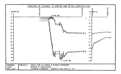
$\frac{\text{Fig. 9}}{\text{of a composite element.}}$  Calculated evolution of the stresses in the upper and lowermost fibre
