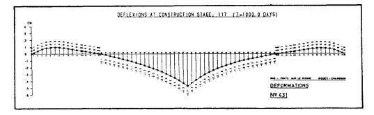
$\frac{\text{Fig. 10}}{\text{stages, from which excess heights of the shuttering can be determined.}}$
