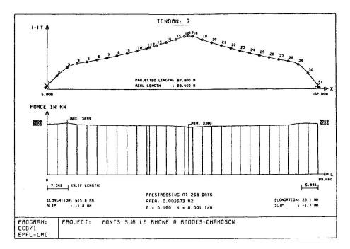
$\frac{\text{Fig. 7}}{\text{of the tendon.}}$  Tendon layout, calculated prestressing forces, and elongations
