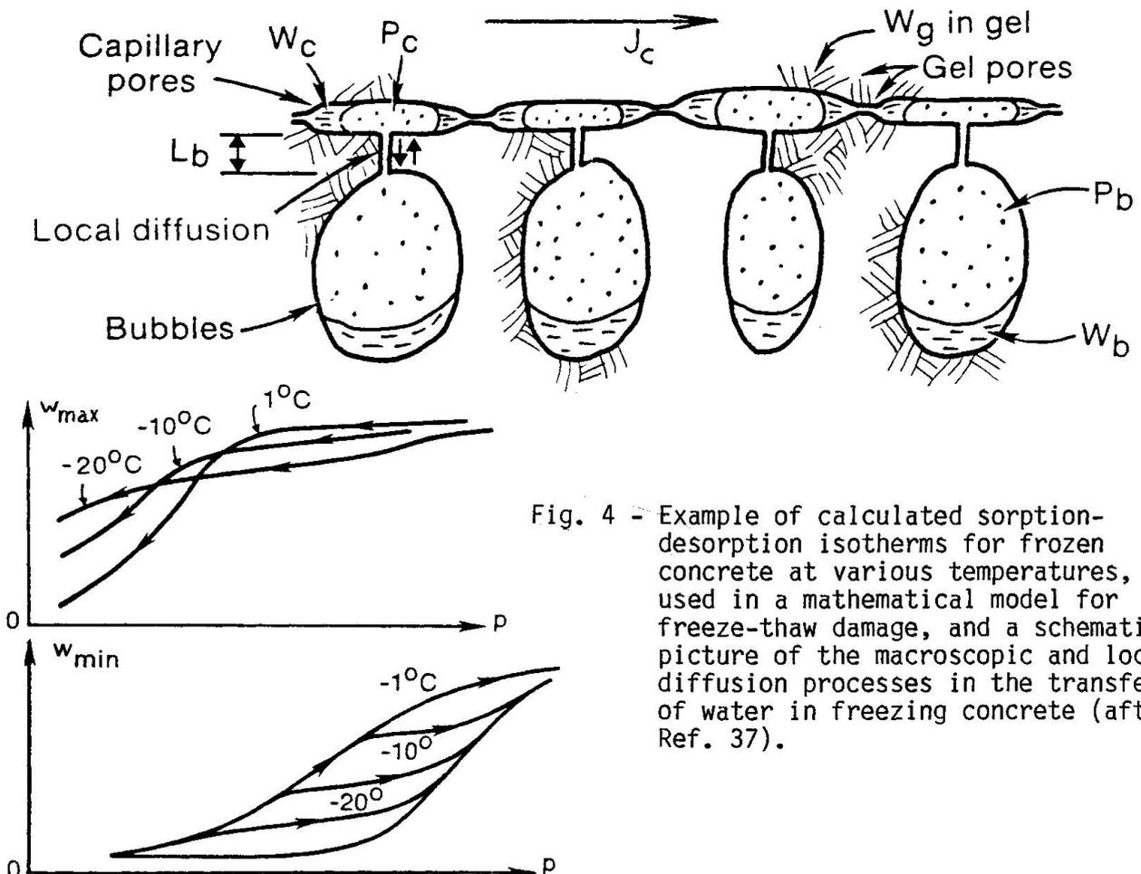
Fig. 4 - Example of calculated sorption-desorption isotherms for frozen concrete at various temperatures, used in a mathematical model for freeze-thaw damage, and a schematic picture of the macroscopic and local diffusion processes in the transfer of water in freezing concrete (after Ref. 37).
