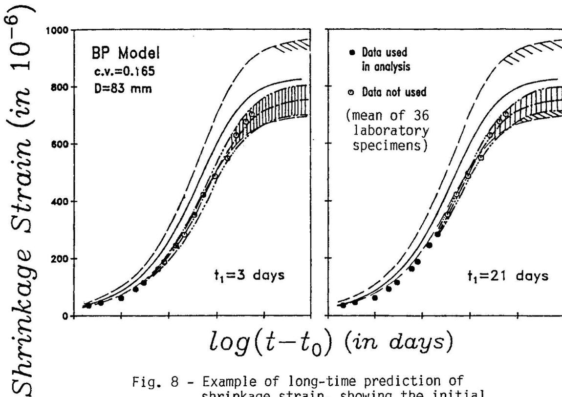
Fig. 8 - Example of long-time prediction of shrinkage strain, showing the initial band of 95% confidence limits and the posterior band after Bayesian updating, based on the solid data point only; after Ref. 35.
