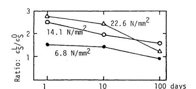
Fig. 15 Ratio between shrinkage under loading  $\epsilon_S^L$  and free shrinkage  $\epsilon_S^0$  as function of duration of drying. Applied external stress is the parameter. (Data after [21]).
