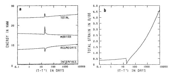
Fig. 18 (a) Distribution of potential energies stored in the components and total stored potential energy as function of duration of loading. (b) Total deformation as function of duration of loading. The temperature is kept constant at  $20^{\circ}\text{C}$  up to (t-t') = 15 days; then the temperature is linearly increased in 12 hours to  $70^{\circ}\text{C}$  and further kept constant.
