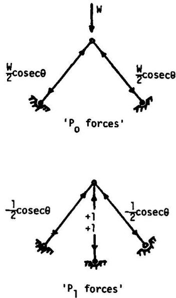
Fig. 5. Loadings on statically determinate released structure.
