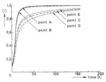
Fig. 7. Development of the maturity r(t) in the corners of the tetrapod.
