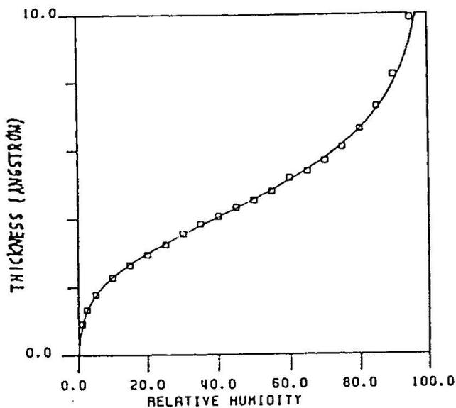
Fig. 1 Physical adsorption on unhydrated cement /1/.
