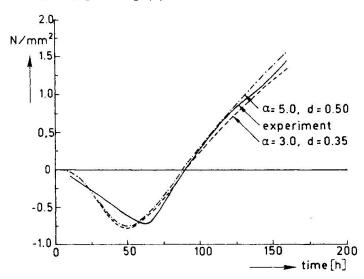
Fig. 3. Calculated stresses with p = 0.30,  $t_0 = 80$ h.,  $\Delta t = 1.0$ h.
