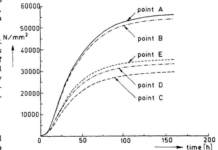
Fig. 8. Development of the stiffness  $E(t)$  in the corners of the tetrapod.
