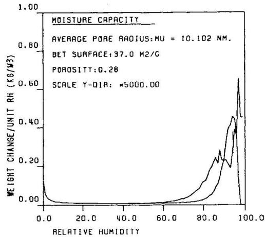
Fig. 7 Moisture capacity.
