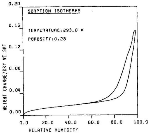
Fig. 6 Calculated sorption isotherm.
