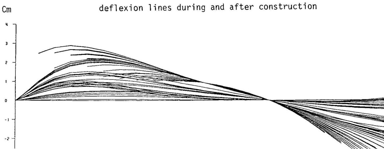
Fig. 8 Detail of a larger computer plot concerning the geometry, tendon layout and calculated deflexion lines.
