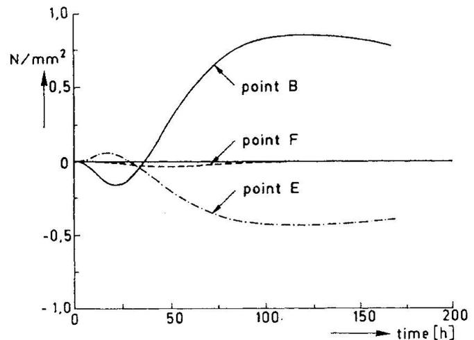
Fig. 9. Stress development  $\sigma_1$  in some points in cross section BE
