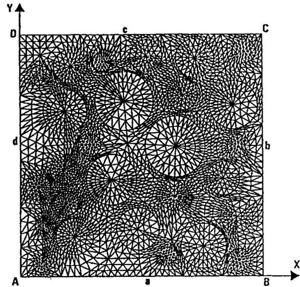
Fig. 3b Finite element idealization of the composite structure used in the analysis.
