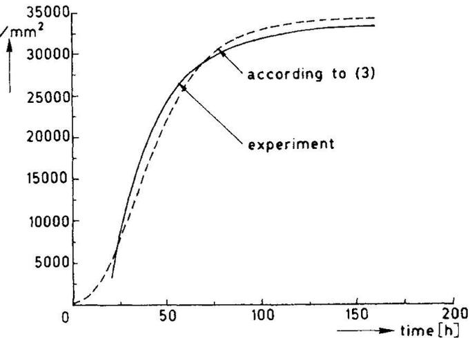
Fig. 2. Development of the stiffness  $E(t)$  according to [6] and eq. (3).
