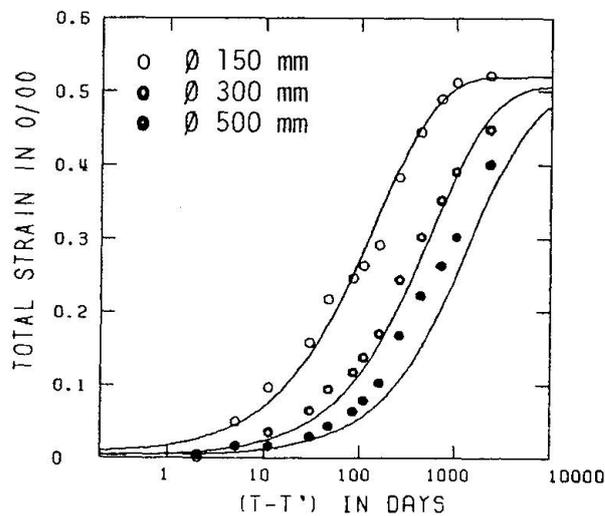
**Fig. 16** Comparison between measured shrinkage strains of cylinders with  $\varnothing$  150 mm, 300 mm and 500 mm, exposed to RH 65%, and calculated shrinkage curves based on a nonlinear diffusion equation and a tensile strain-hardening and softening model with residual strains. Measurements by [1].
