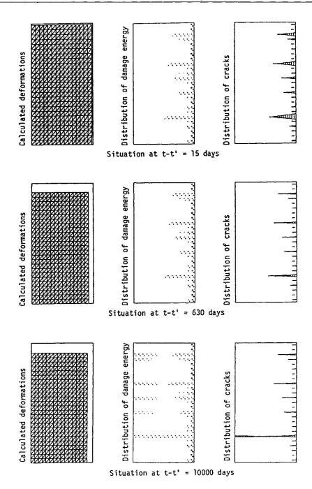
$\frac{\text{Fig. 11}}{\text{colculated deformations, distributions of damage energy and strain}}$  softening at three different durations of drying.
