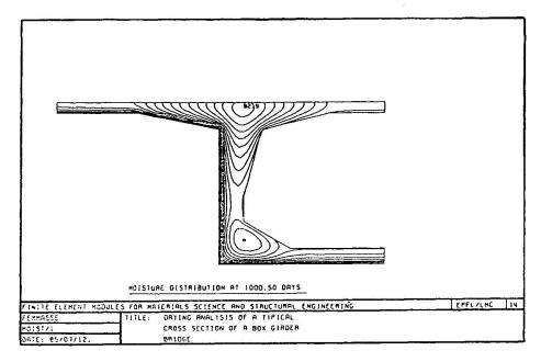
Fig. 3 Calculated moisture distribution 1000 days after demoulding.
