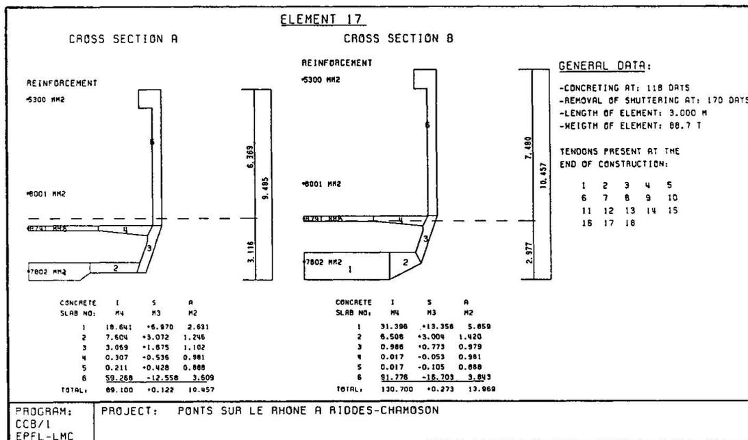
Fig. 6 General information of a composite element in order to check on input data errors.
