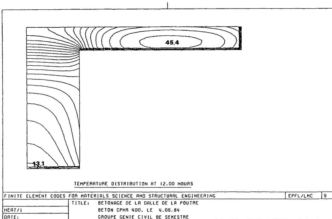
Fig. 1 Calculated temperature distribution 12 hours after concreting.
