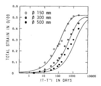
Fig. 16 Comparison between measured shrinkage strains of cylinders with Ø 150 mm 300 mm and 500 mm, exposed to RH 65 %, and calculated shrinkage curves based on a nonlinear diffusion equation and a tensile strain-hardening and softening model with residual strains. Measurements by [1].
