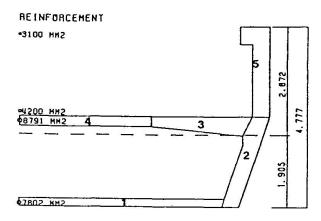
Fig. 11 Division of a cross section in elements.
