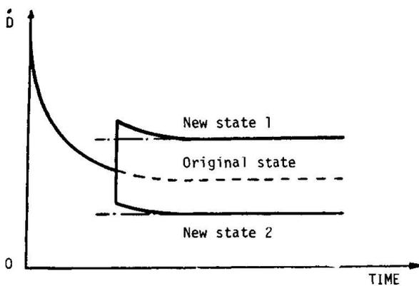
Fig. 3. Changes in Energy Dissipation Rate due to changes of state.
