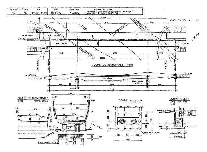
Fig. 5 General situation, cross sections and a longitudinal section of the bridge in construction near Riddes.
