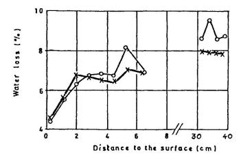
Fig.3: Distribution of residual water content near the skin of the concrete, obtained by drying discs 6-mm thick taken from the structure, at 105°C. It can be seen that the depth of drying did not exceed 50-mm in spite of the age of the structure (11 years).
