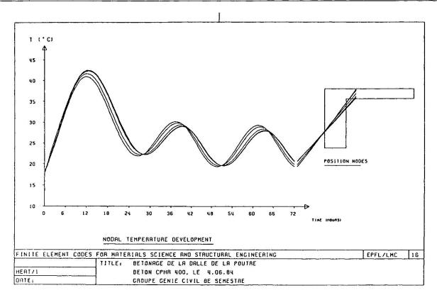
Fig. 2 Calculated development of nodal temperatures.
