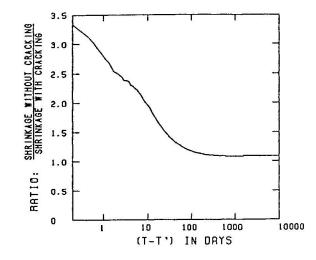
Fig. 12 Calculated shrinkage curves with (a) and without (b) crack formation as function of duration of drying.
