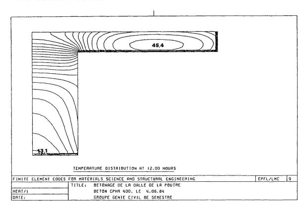
$\overline{\text{Fig. 1}}$  Calculated temperature distribution 12 hours after concreting.
