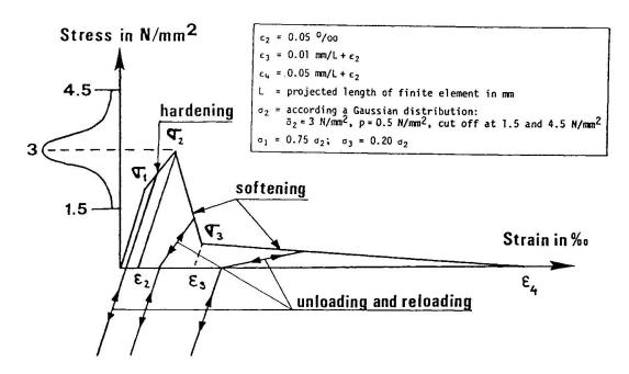
Fig. 10 Strain-hardening and softening model applied in the analyses.
