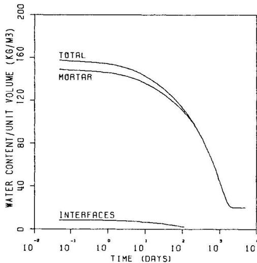
The sharp kink in the curve is due to the convex form of the simulated desorption isotherm mentioned above which is usually not observed experimentally. With a refined model this can be overcome.
