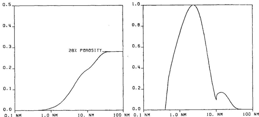
Fig. 3 Cumulative and differential pore size distribution.
