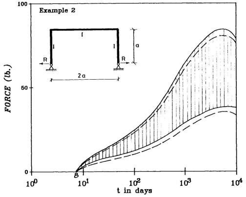
Fig. 6 - Example of a scatter band of mean ± standard deviation (68% probability limits) for shrinkage stresses in a concrete portal frame, obtained by latin hypercube sampling (after Ref. 33).
