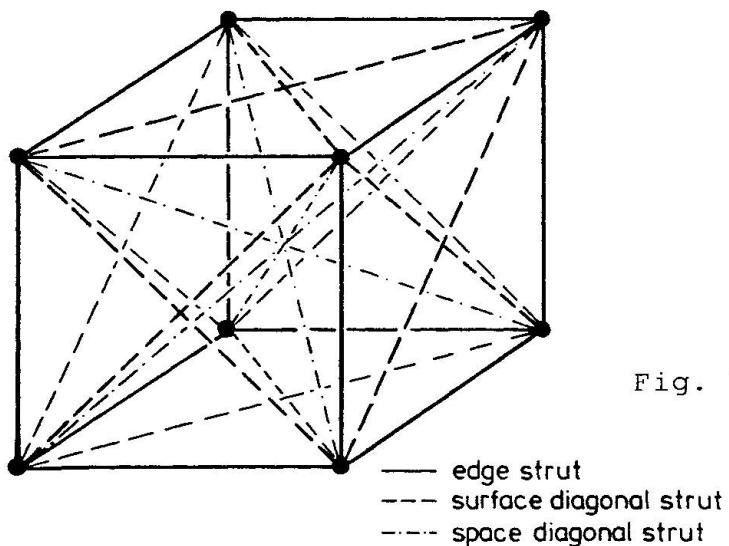
ments may hardly occur. But in heavily degenerated states strut series may buckle or snap through. Thus, a fully geometrically and physically nonlinear analysis of the system has to be performed.
