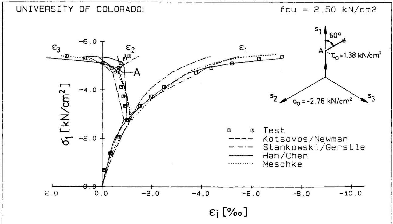
**Fig.8** Nonproportional Deviatoric Load Path after Hydrostatic Preloading
