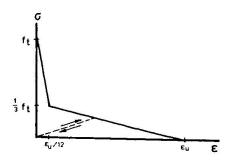
Fig. 4 Bilinear softening diagram.
