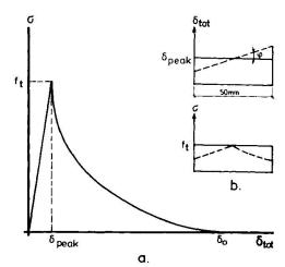
Fig. 3 a) Assumed  $\sigma$ - $\delta$  relation. b) Deformation and stress distributions.
