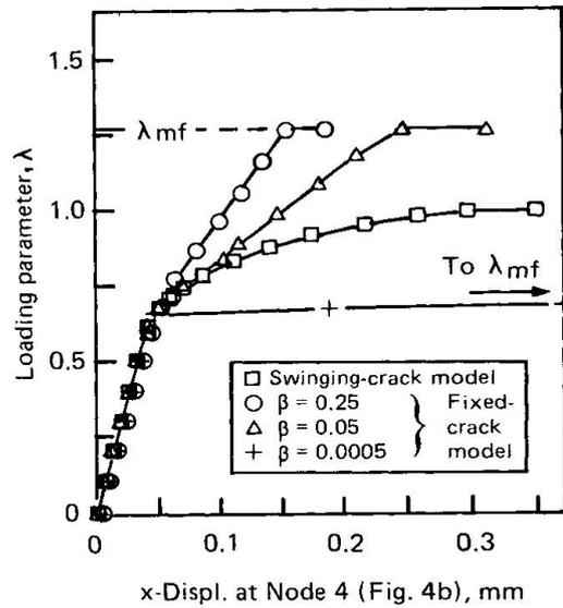
Fig. 6 Influence of shear retention factor,  $\beta$
