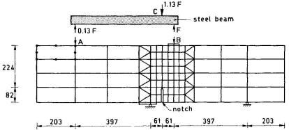
Fig. 4. Element mesh and dimension for unreinforced beam [1].
