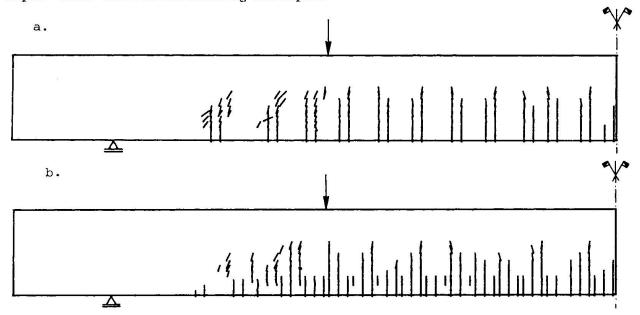
Fig. 10. Crack pattern for reinforced beam.
