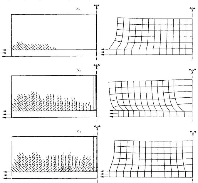
Fig. 3. Tangential crack pattern.
