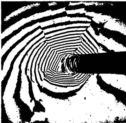
Fig. 7. Localized splitting cracks at end-face, experimentally [3].
