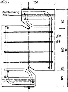
Fig. 1. Push-off specimen used for the shear tests [1,2,3].
