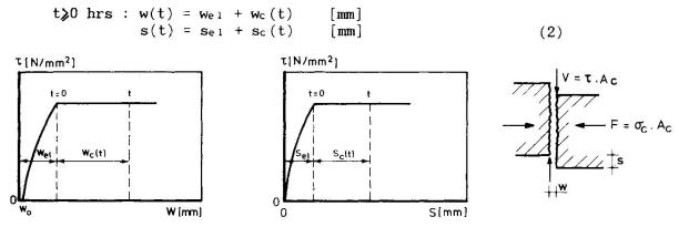
Fig. 3. Definitions of instant and creep displacements as functions of  $\tau$  and t.
