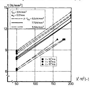
Fig. 10. Development of  $\lambda^4$  as a function of the sustained shear stress  $\tau$ .
