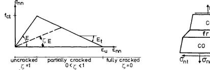
Fig. 11. Tensile stressstrain relation [9].
