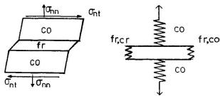
Fig. 12. Rheological model of the fracture zone [9].
