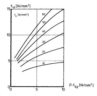
Fig. 2. Static shear strength according to formula (1).
