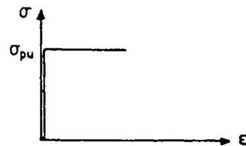
Fig. 8. Rigid-plastic behaviour of matrix material [1].
