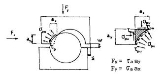
Fig. 7. Contact area between matrix and matrix material [1].
