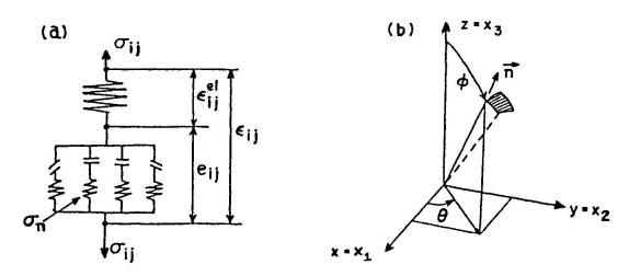
Fig. 1 (a) Rheological Model for concrete (b) Spherical coordinate system.
