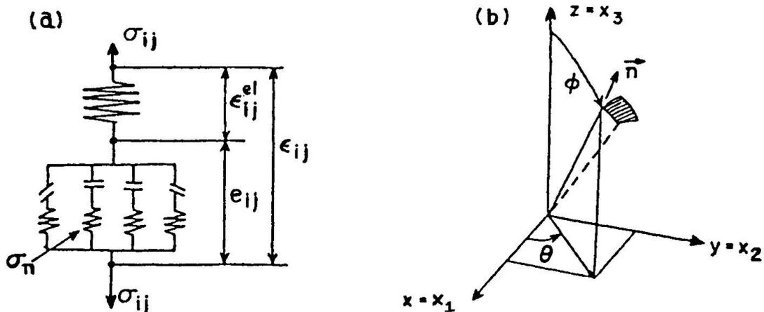
Fig. 1 (a) Rheological Model for concrete
