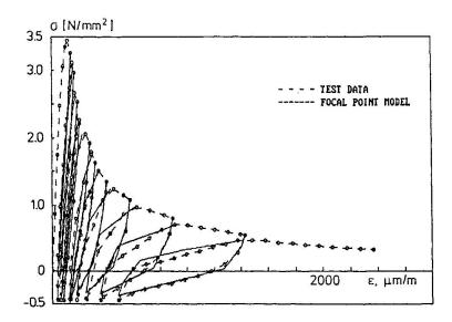
Fig. 6: Comparison with Tensile Cyclic Tests Type III
