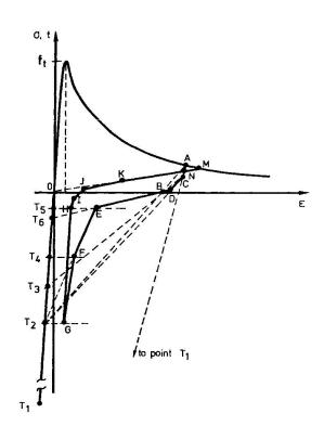
Fig. 2: Focal Point Model for Cyclic Compression
