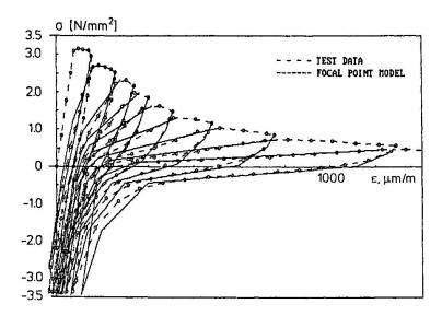
Fig. 7: Comparison with Tensile Cyclic Tests Type IV
