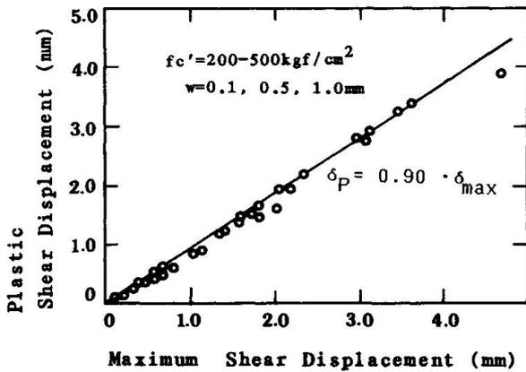
Fig.4 Plastic Shear Component
