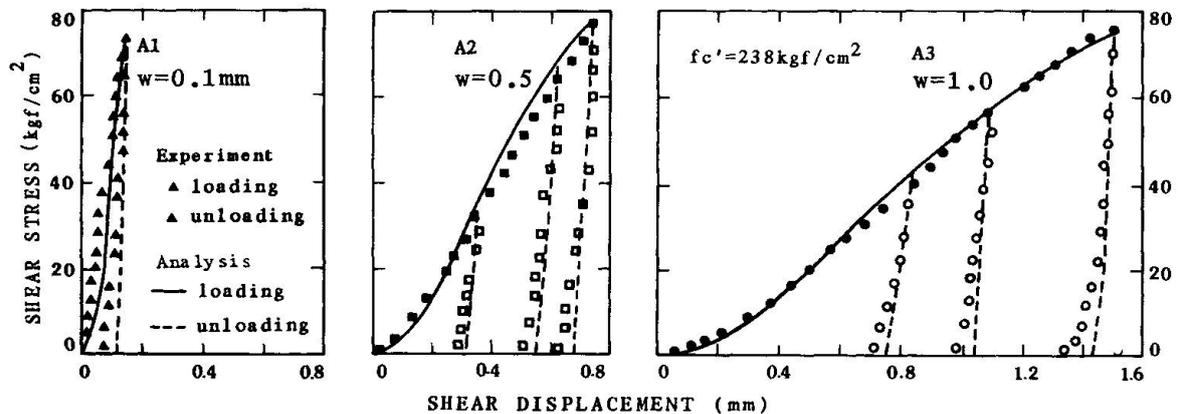
Fig.8 Shear Transfer Stiffness under Various Crack Width
