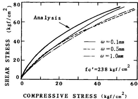
Fig.12  $\tau$ - $\sigma$  Relation under Constant Crack Width
