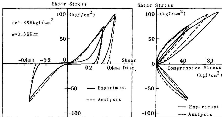
Fig.7 Cyclic Stress Transfer under Constant Crack Width
