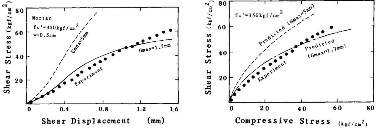
Fig.10 Stress Transfer across a Crack in Mortar
