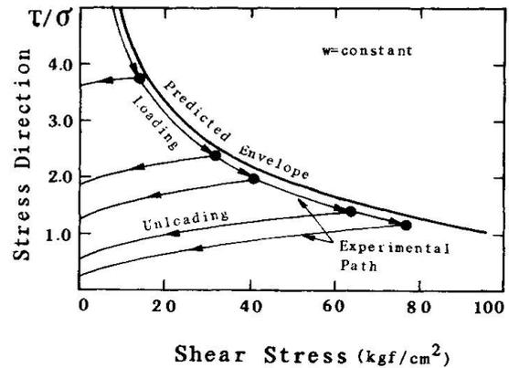
Fig.3 Direction of Stress Transfer under Cyclic Loading
