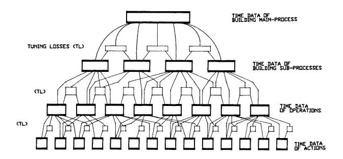
Fig. 6 The ordering of time within a building main-process
