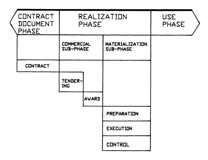
Fig. 2 Project phases, detailed realization phase
