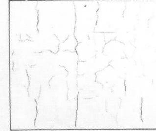
Thin line: Crack width 0.05mm or less / Thick line: Crack width 0.05 - 0.15mm
