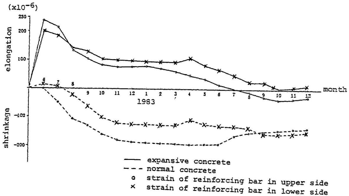
Fig-1 Time-dependent strain variation of reinforcing bar of deck slab in transverse direction.
