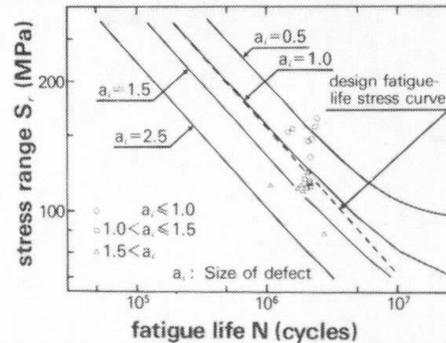
Fig. 1. Predicted  $S_r-N_p$  Curves and Test Results
