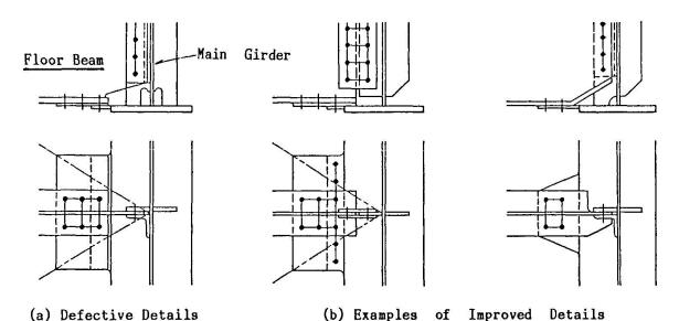
Fig. III Details of Floor Beam
