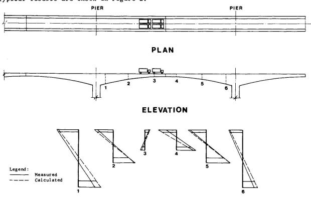
MEASURED AND CALCULATED STRAINS
