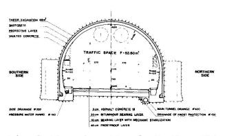
Fig. 2: Tanzenberg Tunnel, Southern Tube Standard Cross-Section with Bays
