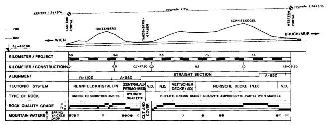
Fig. 1: Tanzenberg Tunnel, Southern Tube - Longitudinal Section
