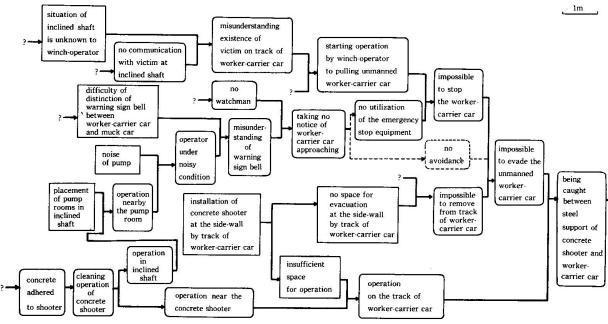
Fig. 3 C.T. diagram of an accident
