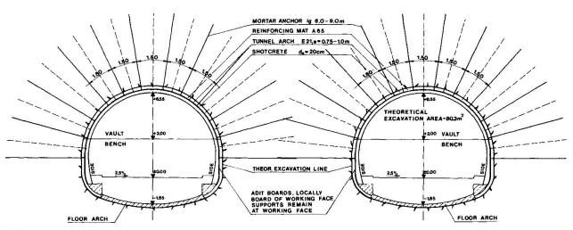
Fig. 4: Bruck Tunnel - Standard Supporting Means in Rock Quality Grade 5
