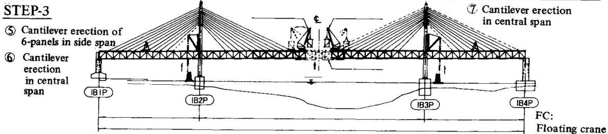
Fig. 3 Illustration of Erection Sequence
