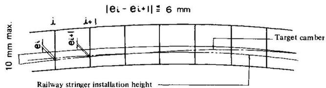
Fig. 6 Railway Stringer Installation Accuracy
