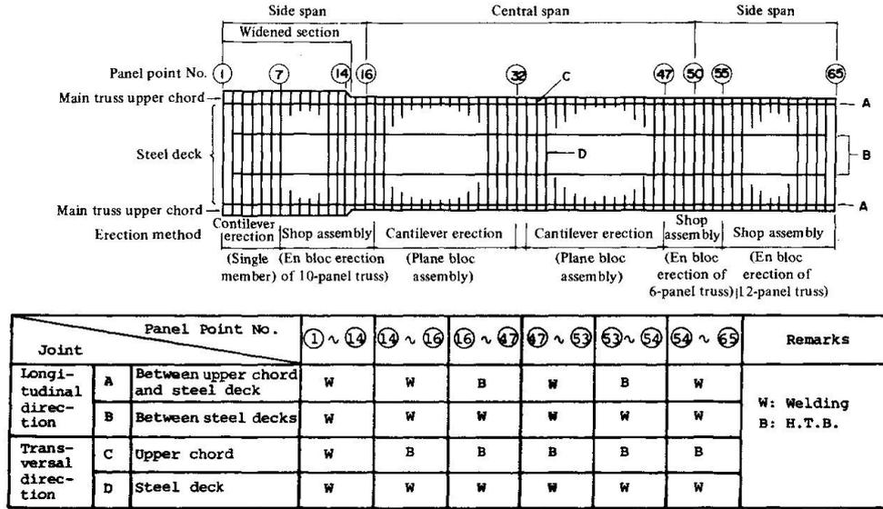
Fig. 4 Classification of Steel Deck Connecting Methods
