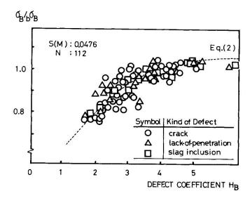
Fig.10 σ<sub>B</sub>/<sub>b</sub>σ<sub>B</sub> versus H<sub>B</sub> Relationship for Butt Joints
