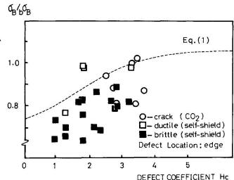
Fig. 8 Test Results of Cross Joints
