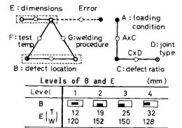
Design of Experiment Fig. 1 ( Test Series I )
