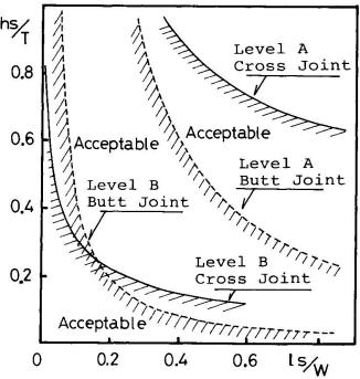
Fig.11 Acceptable Size of Weld Defect
