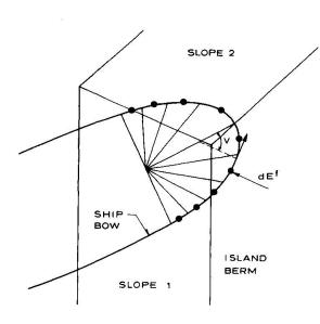
Fig. 3.1 Ship bow discretization
