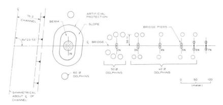
Fig. 2.1 Protection System for the new Skyway Bridge.
