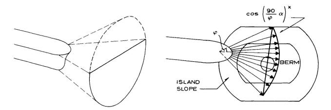
Fig. 4.1 Conical Force Distribution
