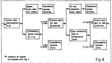
fig. 8 Simple event-tree of scour hole instabilities.
