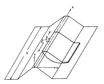
Fig. 1 Geometry of the sliding soil mass (from /3/)
