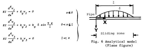
where, E is Young's modulus of the pipe material, I is geometrical moment of pipe inertia,  $\delta$  is maximum displacement of the lateral spreading,  $K_y$  is soil spring constant for transverse motion,  $\mathcal I$  is stretch of the liquefied zone and  $v_1$ ,  $v_2$ ,  $v_3$  are transverse displacements of the pipe.
