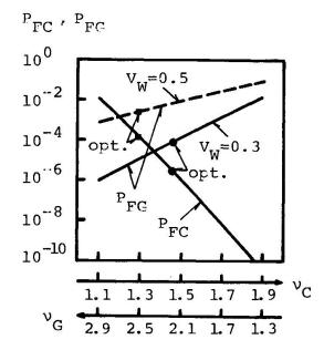
$\underline{\text{Fig.6}}$   $\text{P}_{FC}$  vs.  $\text{v}_{C}$  and  $\text{P}_{FG}$  vs.  $\text{v}_{G}$
