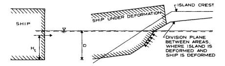
Fig. 3.2 Division Plane with equal Earth Pressure and Ship Strength
