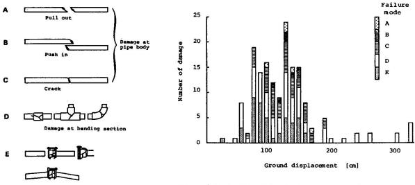
Fig. 3 Failure mode of pipe
