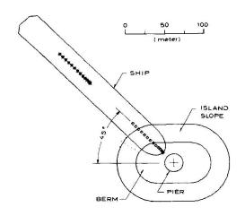
Due to the lifting of the ships bow, only little force is transmitted to the pier in this case.
