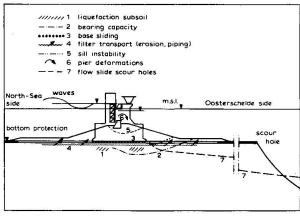
fig. 4 Presentation of the main geotechnical limit states.
