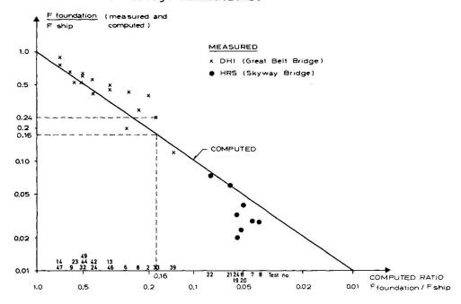
Fig. 5.2 Ratio between Pillar Force and Ship Force in Mathematical and Physical Models
