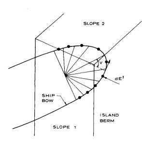
Fig. 3.1 Ship bow discretization
